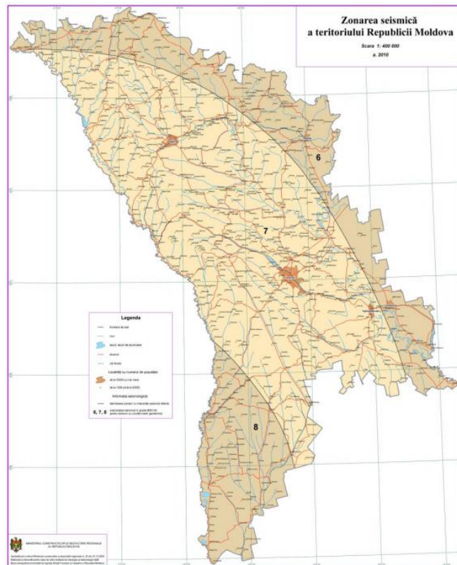
Figure 1 Seismic hazard map of Republic of Moldova in terms of MSK-64
